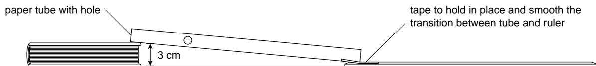
5. Put four small marbles on the middle of the ruler; set one marble on the groove in the center of the ruler, and line up the others on the side towards the tube. Make sure all the marbles are touching. Put the pencil through the holes in the tube, just far enough to block the opening of the tube. Place a fifth small marble in the top end of the tube so that the pencil holds it in place (figure 3).
